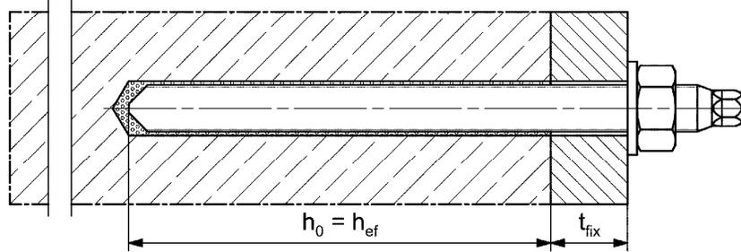
Pre-positioned installation with subsequently injected fischer filling disc:
