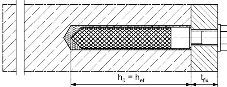
Pre-positioned installation with subsequently injected fischer filling disc:
