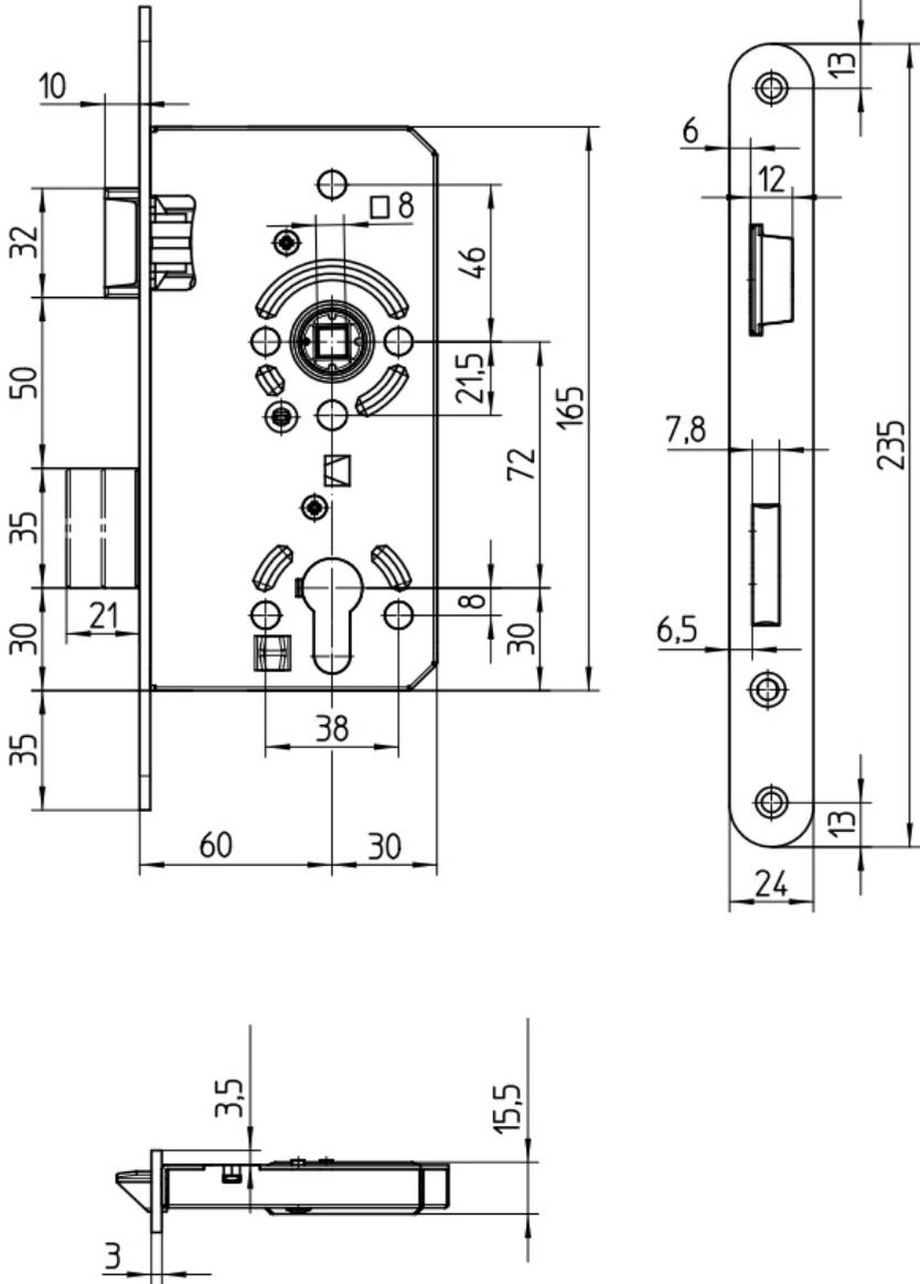
Fixed with 2x chipboard screws 3.5x25mm
