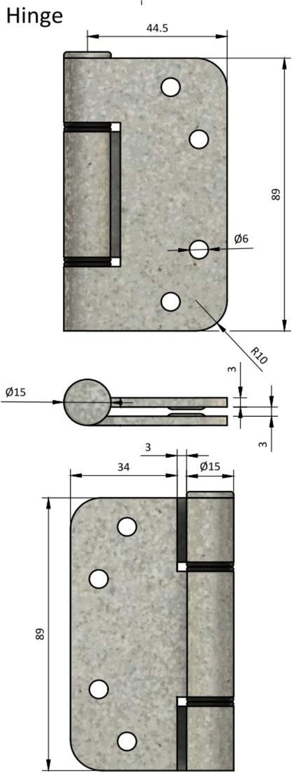
Fixed with 4x chipboard screws 30x3.5mm
