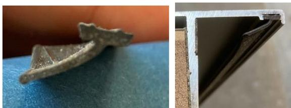
Detailed views of meeting edge seal cross section (left) and mounting position (right)
